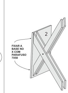
3° PASSO FIXAR A BASE NO X COM PARAFUSO 7X50
