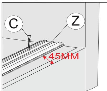
**FIXAR 45MM CONTANDO COM O RODAPÉ PARAFUSO ( D ) 3,5X14MM**
