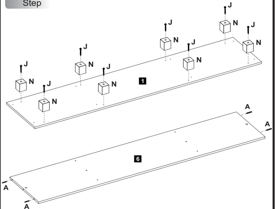
**A** Caviha 04 **J** Parafuso Ø4,0x30mm CP 08 **N** Sapata Square 08
