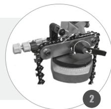
**ALIGN THE GRINDING DISC WITH THE CHAIN TOOTH;**
